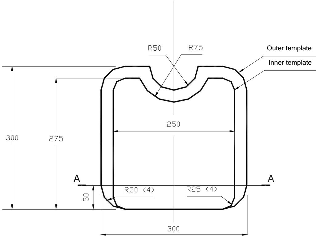
Drawing 3: Cockpit cross section template
